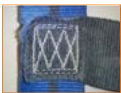
Chest strap damage - tubes slid down against harness creating severe wear
